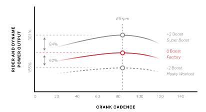
The assist level feature adjusts the output power, which is the percentage of available power put out by the Dyname 4.0 drive system in the different assist modes. There are 4 different modes that can be used to manage battery levels, to adjust trail speed, and to fine tune your effort levels. These modes include: Ludicrous, Trail Plus, Trail, and Eco.
