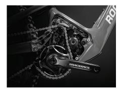
We've removed the upper chain slider that was seen on the Dyname 3.0 drive system to reduce the mechanical noise, as well as the drag when pedalling.
