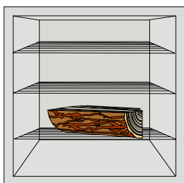
Dry log in a warm oven (105 C) until no further weight loss can be measured.
