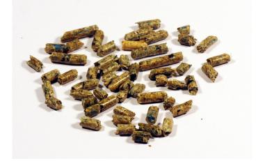
Pellets containing impurities, these have blue plastic amongst other things that should not be in them in them, which can lead to a damaged boiler. Ensure that you only purchase pellets complying to BS EN 1461-2:2011
