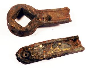
This spanner was found inside a wood chip boiler after it had been chopped into two by the fuel delivery system. Ensure that only wood is fed into the boiler.
