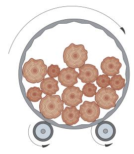
The drum de-barker is a rotating drum that when holding a collection of trunks causes the trunks to abrade against each other and the drum wall to grind off the bark. This system necessitates the logs to be debarked in batches rather than as the continuous flow as with the other systems.
