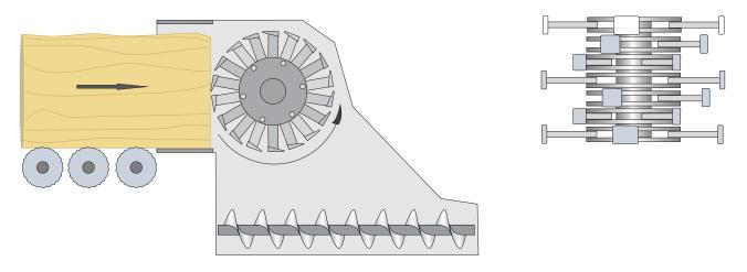
The flail chipper uses blades attached to pivoted arms. These chippers can cope with virtually any size and shape of tree trunk, and because the arms pivot it is almost impossible to stall the cutters. These machines are usually equipped with augers to remove the chips and automatic monitoring controls to ensure the discharge of chips is matched to the supply of wood.
