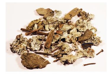
Moulten metal, screws and other metal objects found on the grate of a wood chip boiler. Using pallets to make wood chips is not a good idea.
