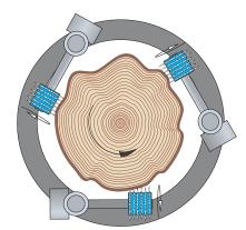
The rosser head de-barker rotates the trunk while it passes a series of pivoting spinning drum cutters.
