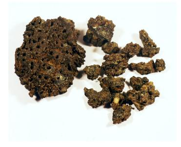
Sintered ash found on the grate of a pellet burning boiler. Only buy good quality pellets and clean out ash from all the combustion areas regularly.
