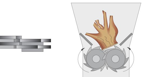
The shredder uses thick closely fitting blades revolving only slowly to rip rather than cut the wood. The design is so successful that these machines are used to shred a wide variety of materials including car bodies and even mattresses. The uncertainty of the chip size uniformity does not make them ideal for chipping wood prior to pellet production but they are used mainly for shredding tree stumps for low grade wood chips.
