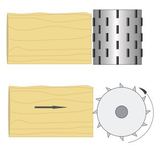
The drum chipper, with whatever blade design it has, produces consistent chip sizes and copes with very large diameter tree trunks and is used by many manufactures of wood chips and pellets. It operates well with straight sided trunks but large and more curvaceous trunks sometimes cause problems when a bulge will split away and stall the drum.
