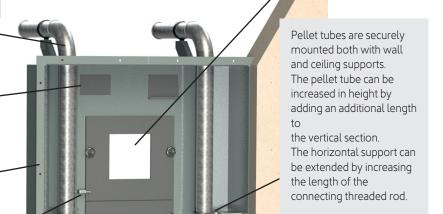
Access doors. The upper door includes the viewing glass and locks the lower door in place. The steel doors can easily be removed to allow access to the fuel store. Each door is held in place by knurled screw knobs.
