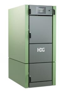
The HDG F Series 50 are down firing gasification split log boilers, it has a 205 litre fuel chamber volume. The logs should be seasoned to 20% moisture content (wet scale).
