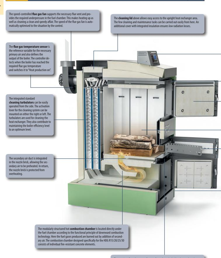
The openings for **primary and secondary air** are locked in place and can be adapted to the particular fuel (hardwood/softwood). The combustion air is supplied through the heating door.
