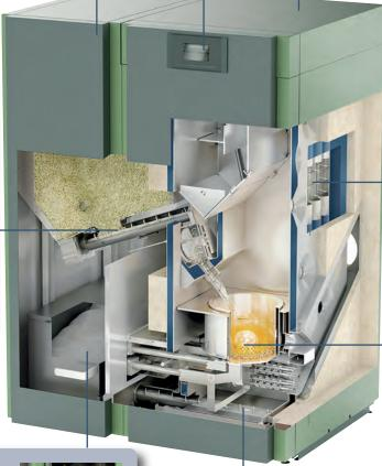
The **fully automatic com- bustion** frees the upright heat exchanger surfaces efficiently of combustion residue. The falling ash is carried away to the external ash container by the fully automatic ash extraction system.
