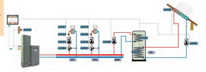
Example 2: For a house with accumulator, two mixed heating circuits and domestic hot water tank, solar thermal system on domestic hot water tank
