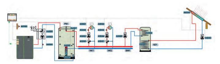
Example 3: For a house with accumulator, two mixed heating circuits, fresh water, dual circuit solar power system
