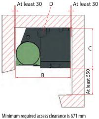
Minimum required access clearance is 671 m Minimum boiler room height 1850 mm
