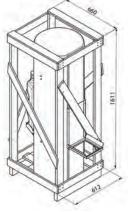
Example packing unit sizes HDG K26 with pellet vacuum feed system
