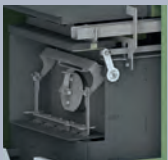
Flue gas flap closed
