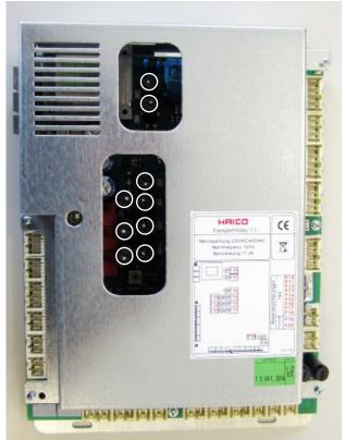
DO NOT use a large screw driver as this can exert too great a force and twist the complete fuse holder from the PCB board so rendering the board useless and this would invalidate any warranty.
