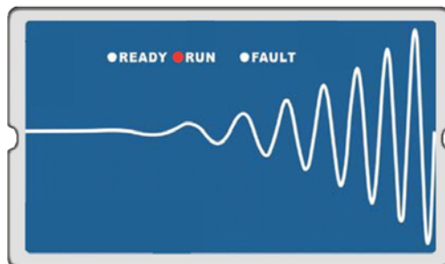
When power is applied, LED „READY“ should light up as shown above.
