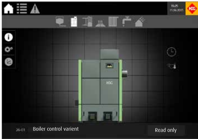
Access to the boiler and heating visualisation and control from any HTML phone, tablet or PC.
