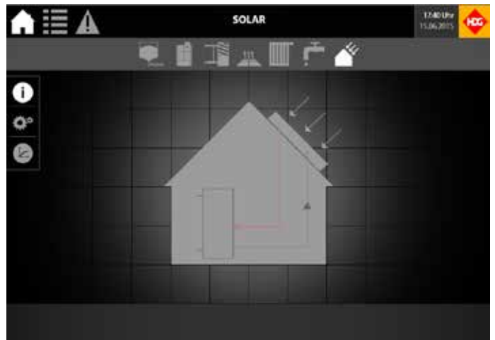
Solar thermal operation can be monitored which can heat up to 3 destinations ie hot water cylinder 1 first, hot water cylinder 2 second, accumulator as a third option.
