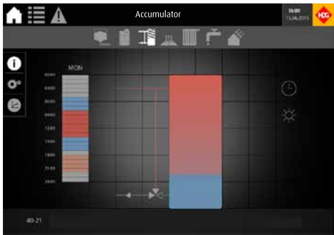
View current heating state of accumulators, change heating start and stops, activate or setup different time clock cycles.
