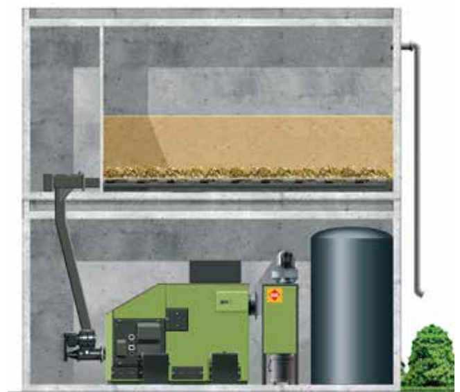
The installation example shows the Pellet delivery system PSZ with HDG Compact 200 and HDG cyclone dust separator
