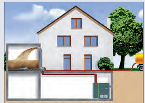
Example: Fuel storage remote to the boiler. Pellets transported to the boiler by vacuum system.
