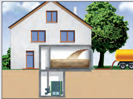
Example: Pellet storage with blown delivery
