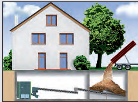
Example: Transport of fuel from a distant fuel storage via a second auger.
