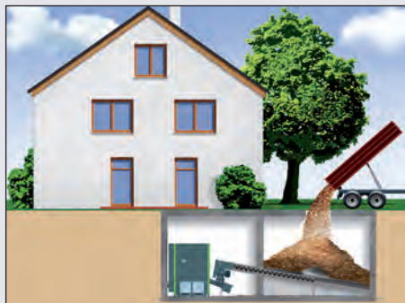
Example: Fuel storage underground with above-ground access hatch
