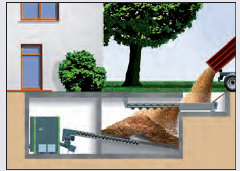
Example: Fuel storage in the basement with a cross auger to move fuel.
